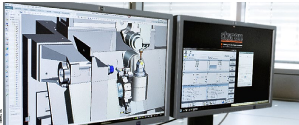
Example of a CAD/CAM CNC process chain using NX and Sinumerik VNCK (Chiron ProcessLine)
